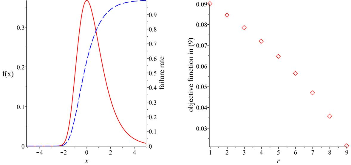
Figure 1: Gumbel distribution with parameter 1. *Left*: Pdf  $f(x)$  (solid line, left scale) and failure rate  $\frac{f(x)}{1-F(x)}$  (dashed line, right scale). *Right*: The objective  $\bar{\beta}_{r,n}$  for  $n = 10$  is maximized at  $r^* = 1$ .
